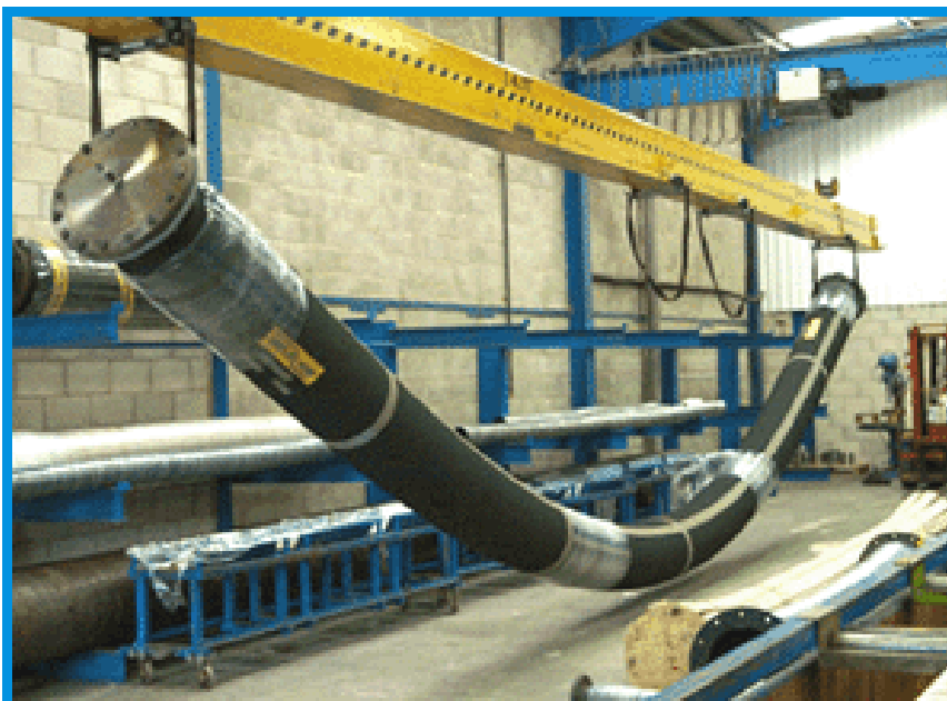
Above: 16" id dredger discharge hose with integral fixed flanges.
